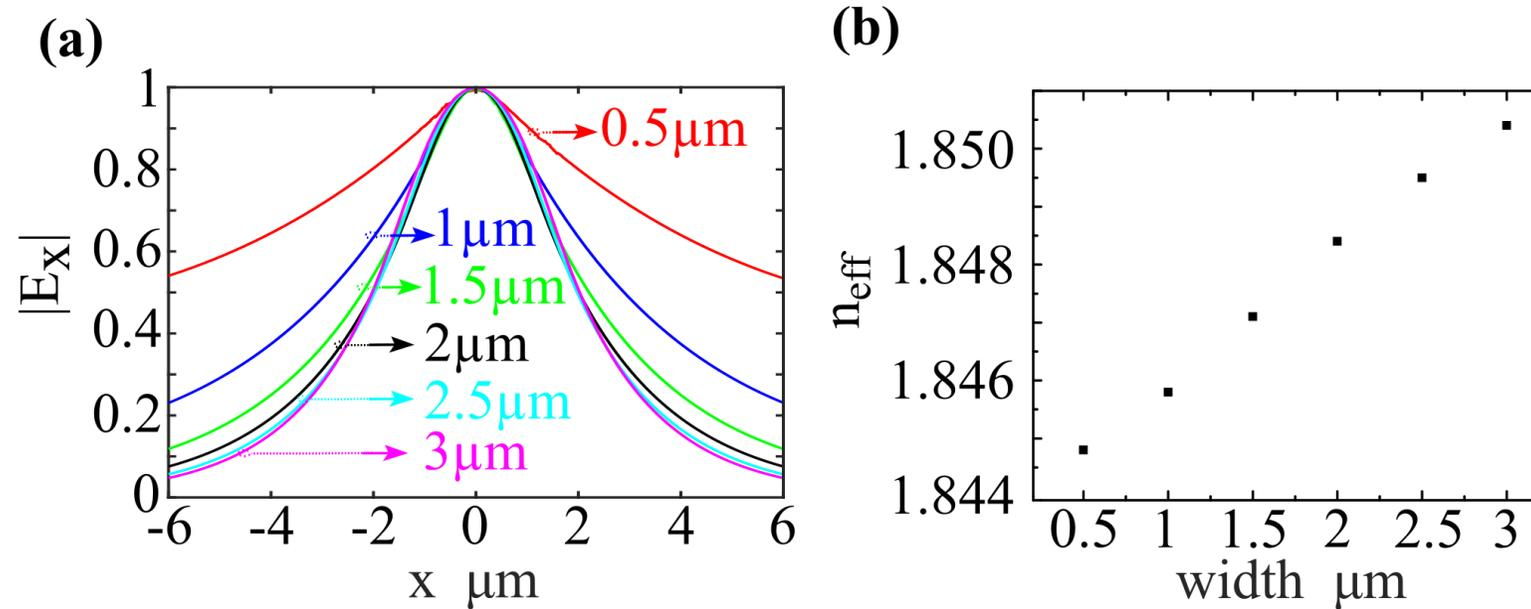
**Figure 15:** Quasi-TE polarization.  $|E_x(x, y)|$  modes are normalized to the maximum amplitude while varying the width of the strip in the strip-loaded waveguides. The indicated values represent the cross-section profiles (a) and the change in the effective mode index (b) of the waveguide width with the strip width from A. Katiyi and A. Karabchevsky 2017.
