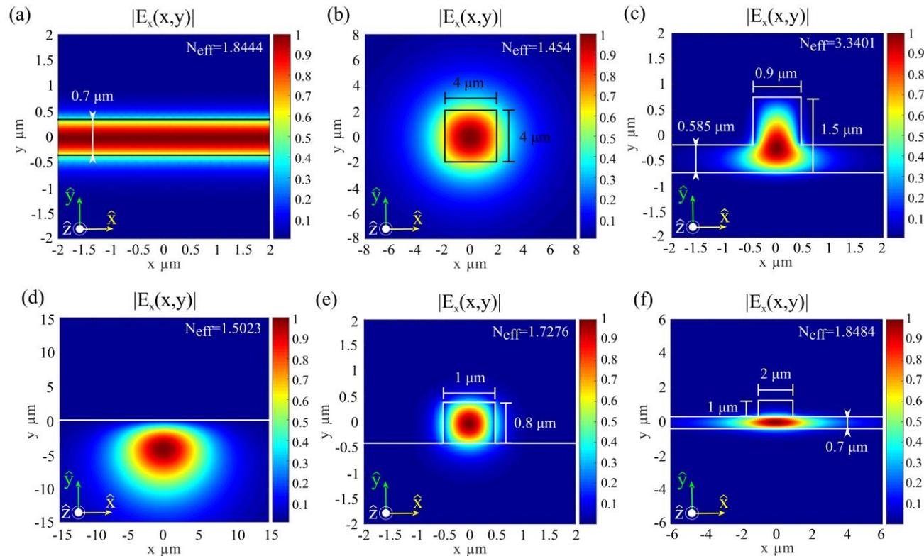
**Figure 13:** Quasi-TE polarization. Colormaps of  $|E_x(x,y)|$ , normalized to the maximum amplitude in single-mode waveguides: (a) slab, (b) buried, (c) rib, (d) diffused, (e) ridge, and (f) strip-loaded from A. Katiyi and A. Karabchevsky 2017.
