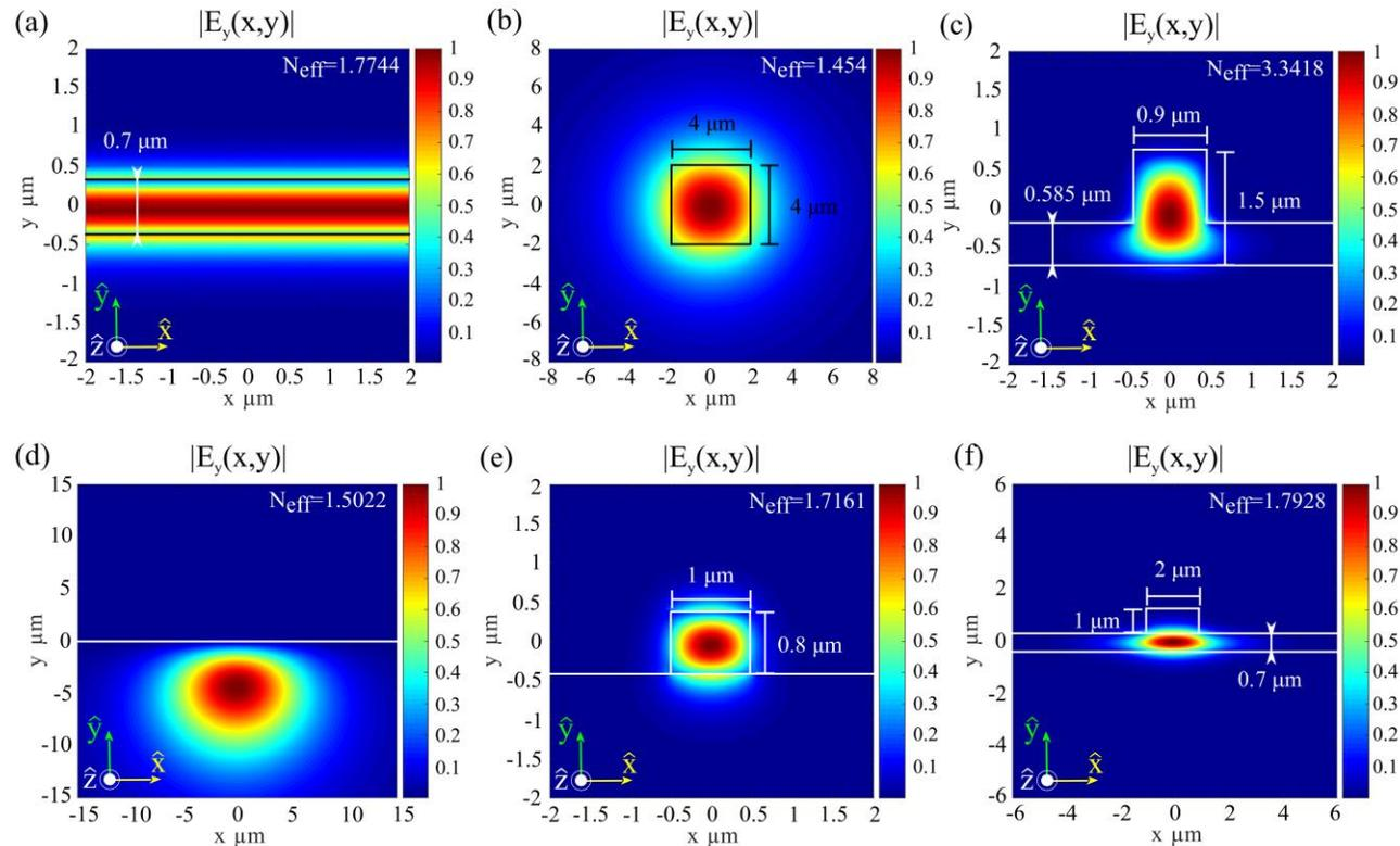
**Figure 14:** Quasi-TM polarization. Colormaps of  $|E_y(x,y)|$ , normalized to the maximum amplitude in single-mode waveguides: (a) slab, (b) buried, (c) rib, (d) diffused, (e) ridge, and (f) strip-loaded from A. Katiyi and A. Karabchevsky 2017.
