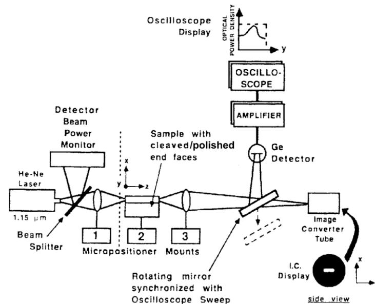
**Figure 9:** Diagram of an experimental setup that can be used to measure optical mode shapes.
