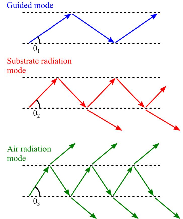
Figure 6: Diagram of the possible modes in a slab waveguide
