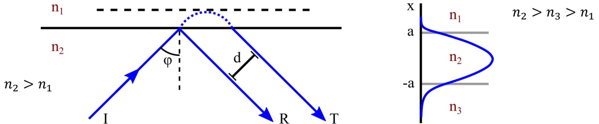
**Figure 4:** Total internal reflection and Goos-Hänchen shift.  $R$  is the behavior of the partially reflected beam,  $T$  is the behavior of the total internal reflection beam and  $d$  is the Goos-Hänchen shift.
