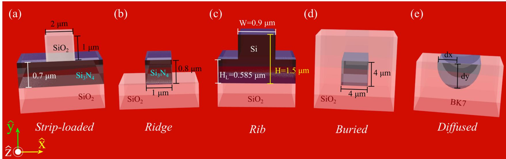
**Figure 12:** Common laterally confined passive waveguide structures: (a) a strip-loaded waveguide made of nitride on a silica substrate covered by silica, (b) a ridge waveguide made of nitride on a silica substrate, (c) a rib waveguide made of silicon on a silica substrate, (d) a waveguide buried in silica glass, and (e) a diffused waveguide in borosilicate glass from A. Katiyi and A. Karabchevsky *Lightwave Technology* 35:14, 2902 - 2908, (2017)
