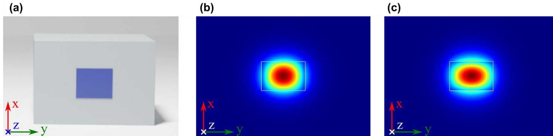
**Figure 5:** (a) Illustration of a buried waveguide. The field distribution of (b) transverse electric (TE) fundamental mode and (c) transverse magnetic (TM) fundamental mode of buried waveguide with dimensions of  $1 \times 1.5 \mu\text{m}$ .
