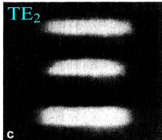
Optical mode patterns in a planar waveguide, a TE<sub>0</sub>, b TE<sub>1</sub>, c TE<sub>2</sub>. In the planar guide, light is unconfined in the y direction, and is limited, as shown in the photos, only by the extent of spreading of the input laser beam.
