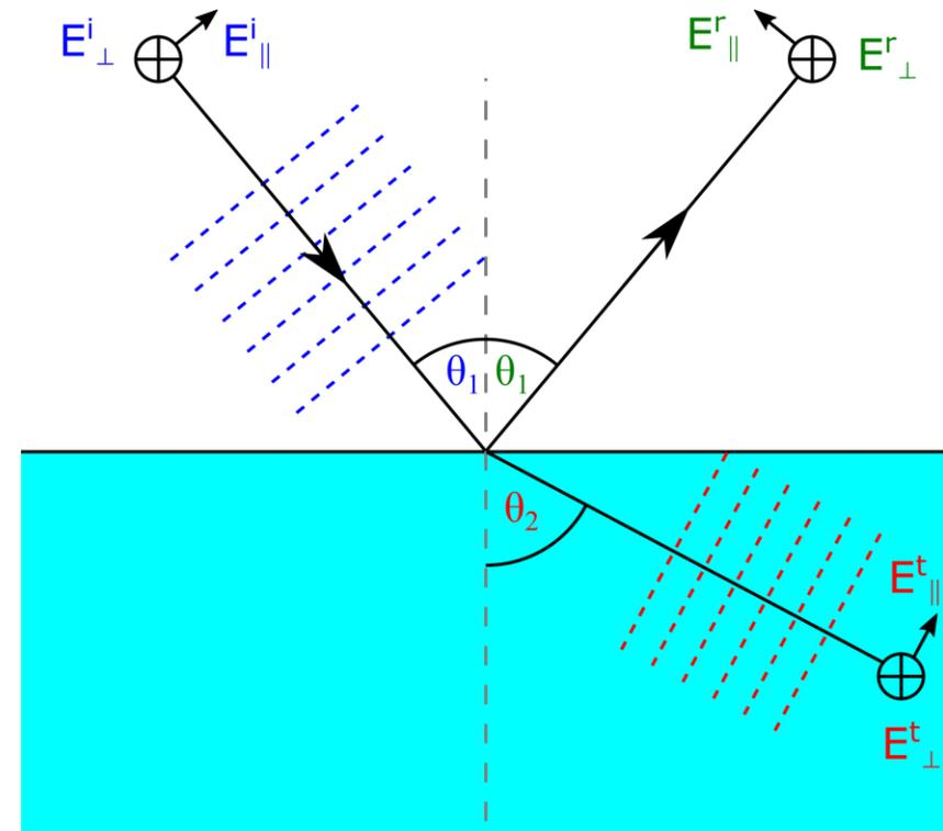
Figure 2: Plane wave reflection and refraction at an optical interface.
