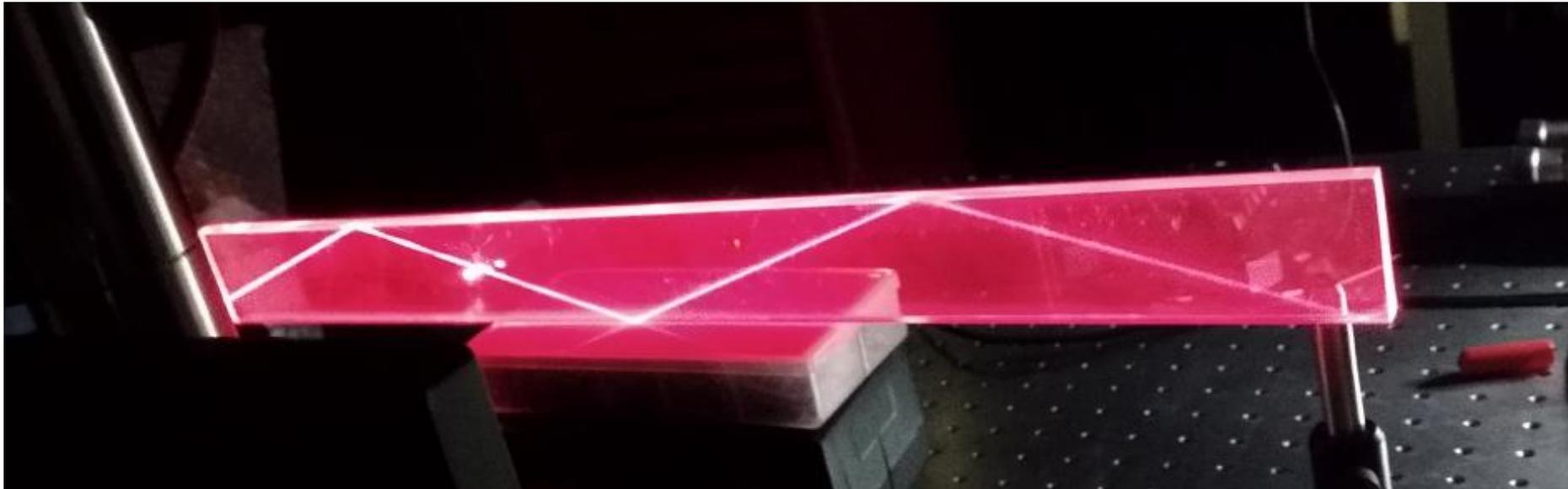
**Figure 1:** A laser beam through acrylic shows the concept of total internal reflection (the light doesn't continue straight through the edge of the glass but bounces back and forth until exiting at the end).
