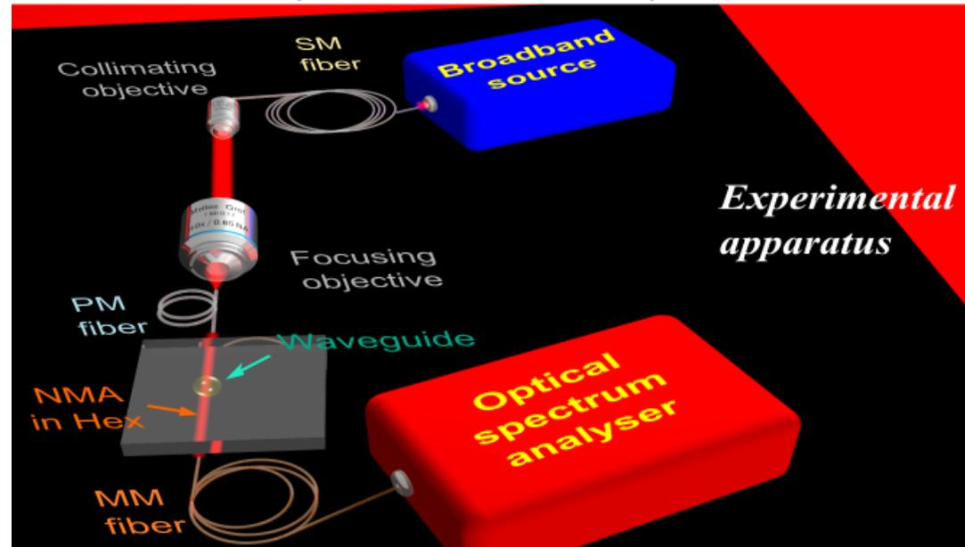
Figure 10: Butt-coupling to a channel waveguide.
