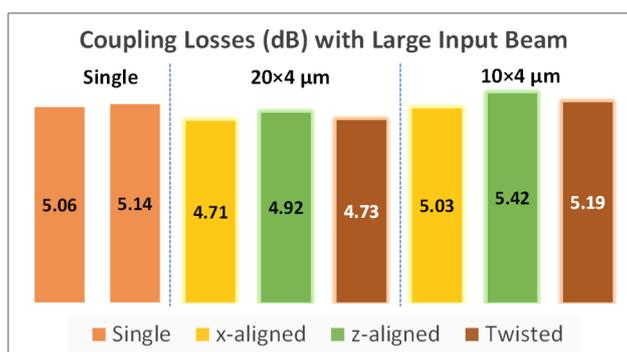
Figure S6. Coupling losses of the waveguides from an expanded Gaussian input beam with diameter of  $\sim 13.2\mu\text{m}$  at 785 nm wavelength. The detailed waveguide cross-sections are described in Fig. 3 (a) of main text.
