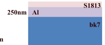
3. Positive photolithography hard mask UV exposure
