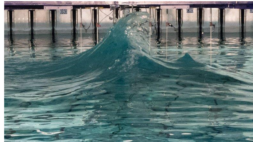
Recreation of the Draupner wave in a circular wave tank [2].
