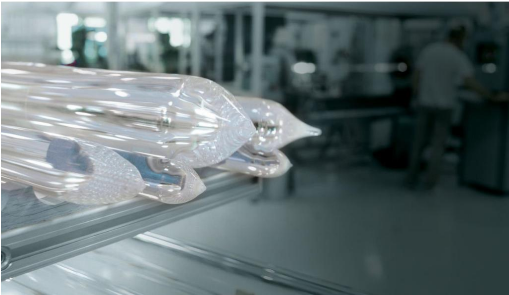
Figure 6: (a) Fiber preform [from LEONI fiber optics]. (b) Fiber special preform [from kohokukogyo]
