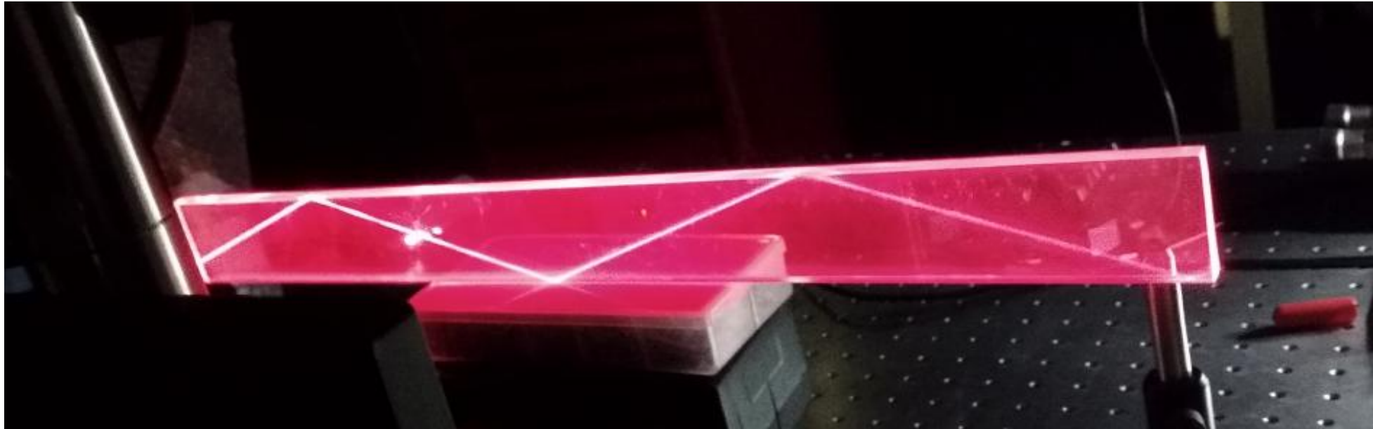
Figure 16: A laser beam through acrylic shows the concept of total internal reflection (the light doesn't continue straight through the edge of the glass but bounces back and forth until exiting at the end).
