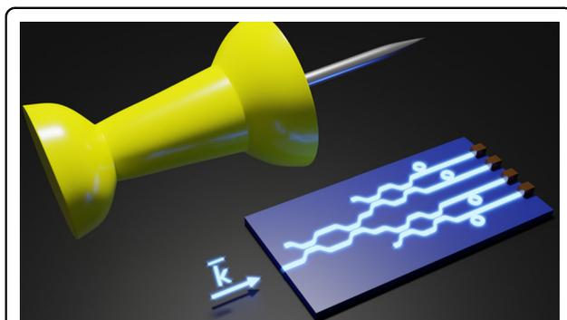
**Fig. 1** The schematic view illustrates an ultra-tiny spectrometer designed to fit on a microchip. For scale comparison, the device is shown alongside a thumbtack. The direction of the light is indicated by the vector  $k$
