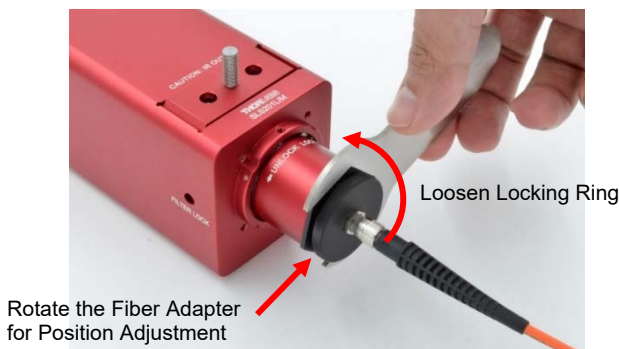
Figure 11 Adjust Fiber Adapter Position
