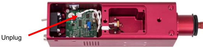
Figure 17 Unplug the bulb module connector.
