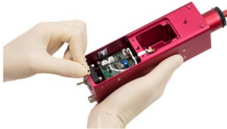
Figure 16 Loosen the bulb module locking screw.
