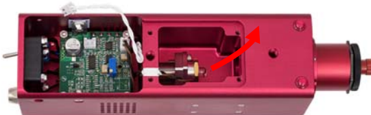
Figure 18 Pull out the bulb module.
